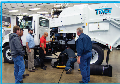
Attendees review components of the pick-up head assembly during removal and installation.
