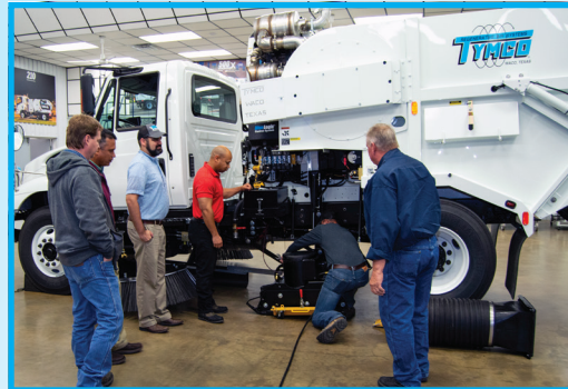
Attendees review components of the pick-up head assembly during removal and installation.
